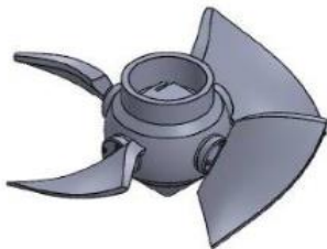
Fig. 6: 3D View of runner blade
